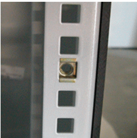
Figure 5: Kiosk frame with nut (left picture) for the lower PC bracket (installed, right picture).
